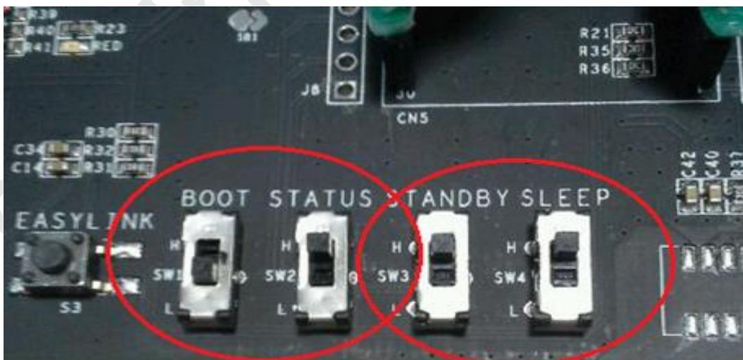
Figure 14 Development Board Switch Settings
